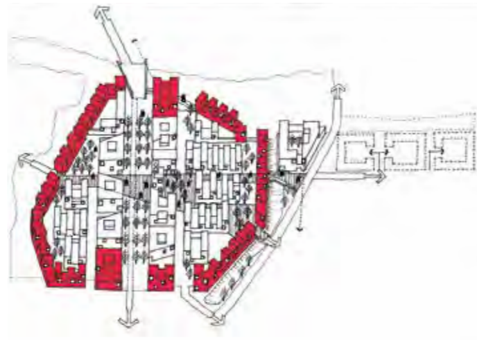
Concept sketch showing defined settlement edge of a new neighbourhood at Northstowe, Cambridgeshire
